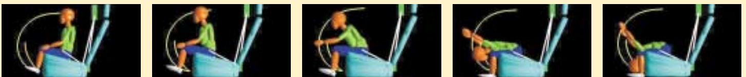
6-year-old child dummy, scooted forward in seat, restrained by the lap belt only. 35 mph crash. Extensive dummy movement.
