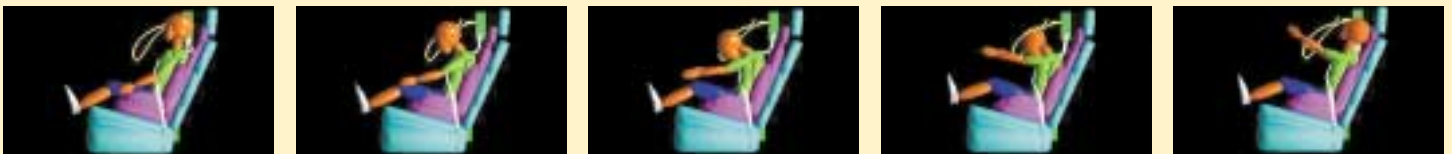
6-year-old child dummy in a belt-positioning booster seat, restrained by a lap-shoulder belt. 35 mph frontal crash. Little dummy movement.
