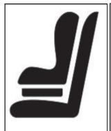
Booster seats are intended to provide a platform that lifts the child up off the vehicle seat in order to improve the fit of the child in a three-point adult safety belt. The seat should also position the lap belt portion of the adult safety belt across the child's hips or pelvic area. An improper fit of an adult safety belt can cause the lap belt to ride up over the stomach and the shoulder belt to cut across the neck, potentially exposing the child to serious abdominal and neck injury.
