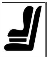
Booster seats are intended to provide a platform that lifts the child up off the vehicle seat in order to improve the fit of the child in a three-point adult safety belt. The seat should also position the lap belt portion of the adult safety belt across the child's hips or pelvic area. An improper fit of an adult safety belt can cause the lap belt to ride up over the stomach and the shoulder belt to cut across the neck, potentially exposing the child to serious abdominal and neck injury.
